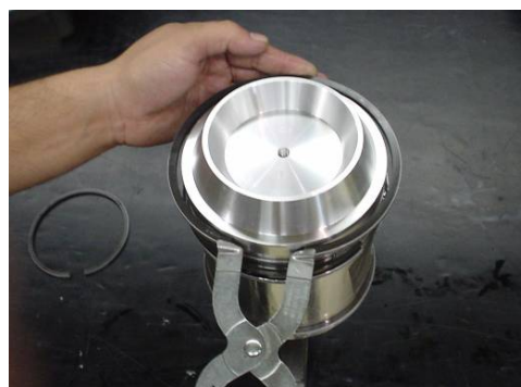
Piston ring removal tool
