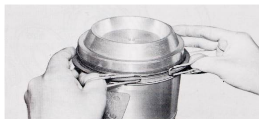
Piston ring removal tool
